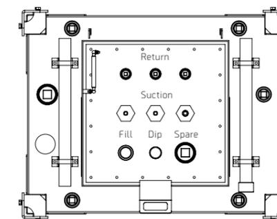
TYPICAL INNE TANK CONFIGURATIONS
